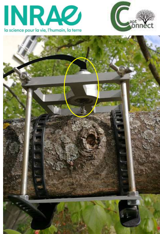
Tree measurement thickness device with D03 Transducer (mounted on top). Maintained by INRAE, a French Laboratory. ( INRAE, l'Institut national de recherche pour l'agriculture, l'alimentation et l'environnement | Ministère de l'Agriculture et de l'Alimentation ) Manufactured by Capt. Connect. High resolution means even slightest growth can be tracked.
