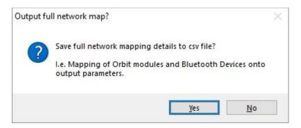
Selecting yes will provide a CSV file describing the external parameter mapping onto modules and Bluetooth channels, an example is shown below: -
