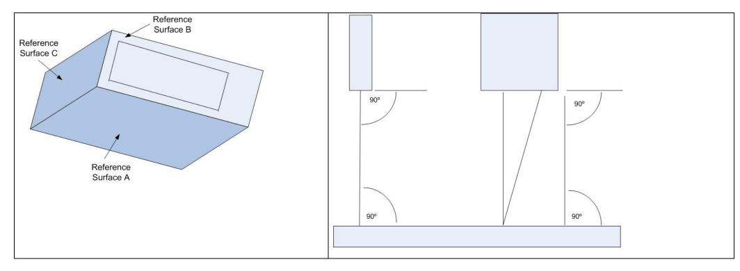
When mounting the head the goal is to have the Reference Surface B parallel as possible to the plane of the target. Take care when using mechanical blocks etc to set up the laser as the window may be scratched. Measurement Set Up
