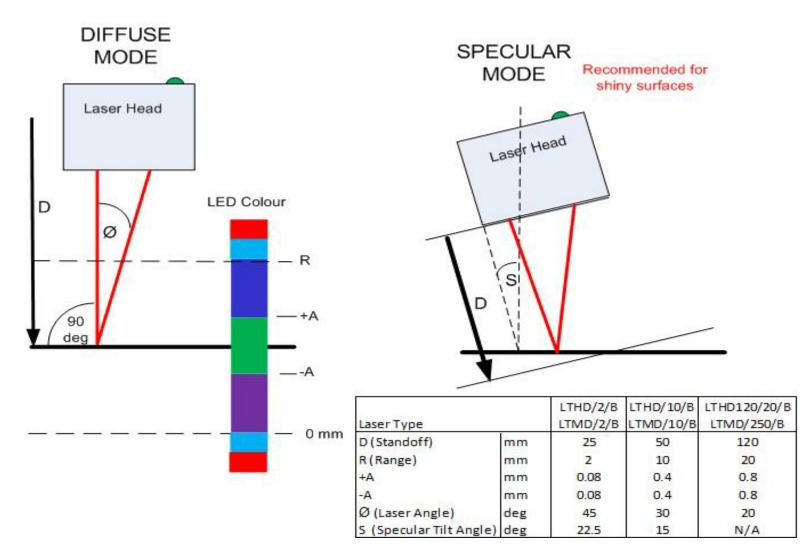
The green led indicates the most accurate position for measurement.
