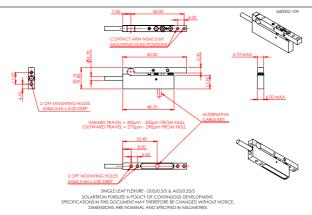
Shown is the Solartron Single Leaf Flexure - refer to Solartron website for latest drawing.
