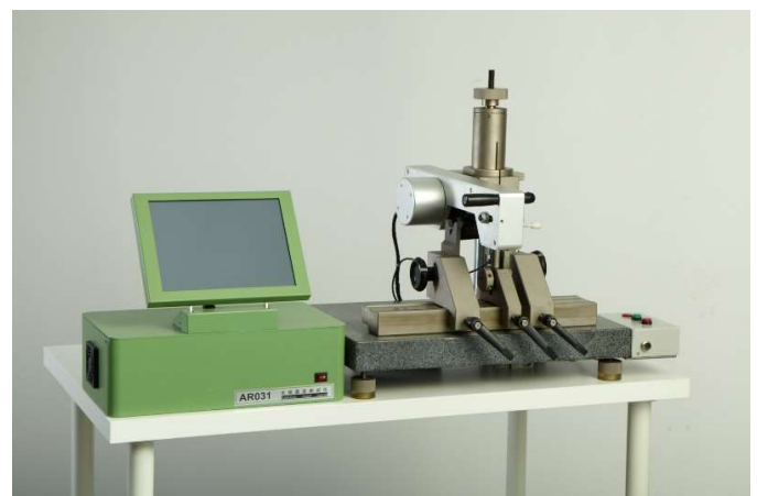
Shenzhen Zhuidian (SZ) in China uses an AXR/1/S to check the runout and TIR of rotor blades.
