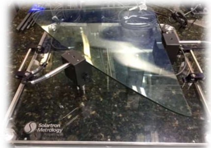
Feather Touch probes are often used to check Automotive Glass
