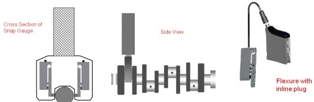
In the event the Single Leaf becomes damaged from misuse, it can quickly be changed out with an optional Digital Inline Plug. With this feature, all calibration data is loaded into a chip inside the plug (competitors use a potentiometer for mapping data, which is susceptible to drift). Once connected to a PIE module, Orbit® 3 instantly recognizes the probe or flexure, and gauging can continue with little downtime.
