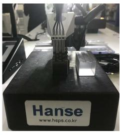
3mm probes checking different ridges.
