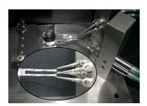
Lever Probes checking several points on an HDD component
