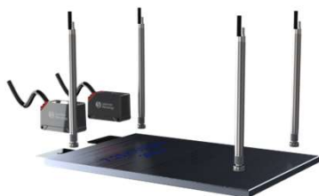
Orbit LT Lasers and Digital probes gauging a Battery Cell
