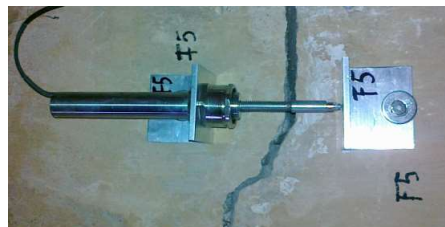
S-series transducer monitoring a crack
