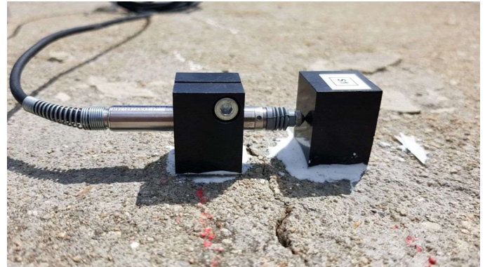
Solartron gauging probe monitoring a crack
