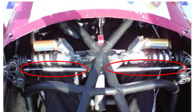
Solartron displacement transducers mounted to the interior of a race car frame
