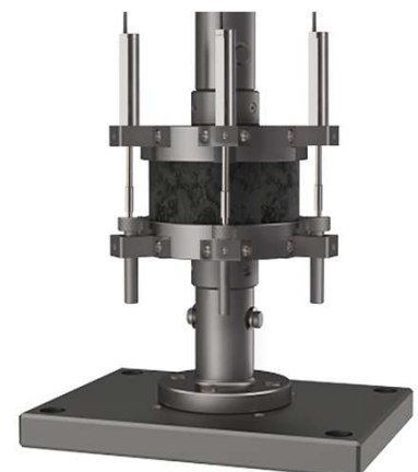
Measurement of concrete compression
