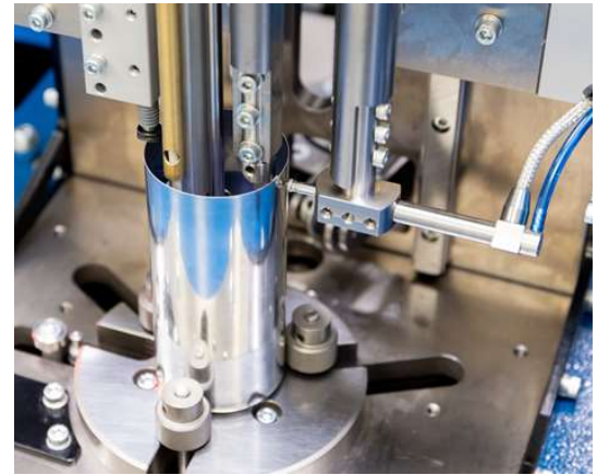
One probe is checking height of an aluminum can, while another checks thickness
