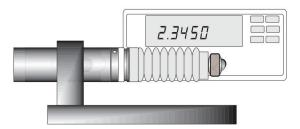
1) Before opening the transducer, a reference reading needs to be taken with the probe tip fully extended. Remove the transducer from the power source.
