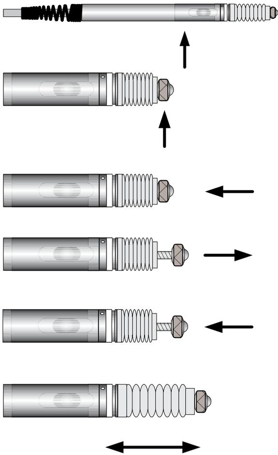
1) Hold the transducer body firmly in the hand or with a pair of soft jaw pliers (to prevent damage to the transducer body).
