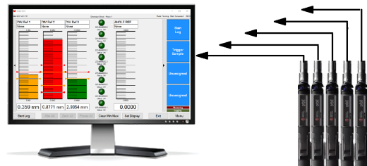
Static Mode (above) vs. Read Burst Mode (below). With Read Burst, readings from all modules sent simultaneously
