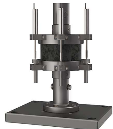
Measurement of concrete compression
